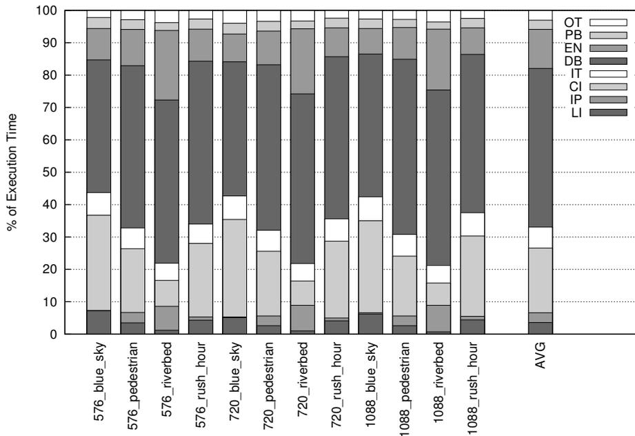
Figure 2: Profiling of H.264 Decoder with AltiVec Optimizations.
