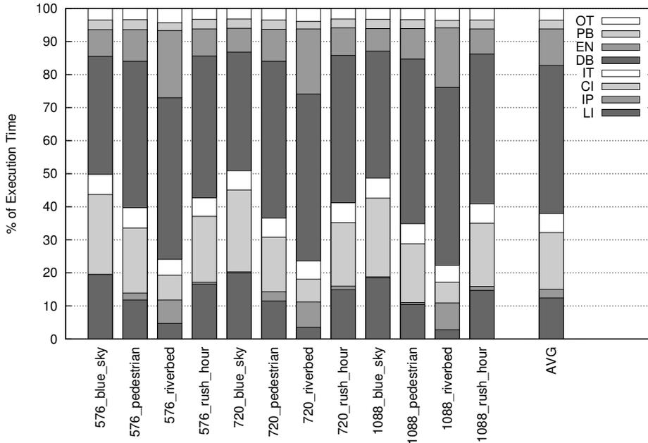
Figure 1: Profiling of H.264 Reference Decoder
